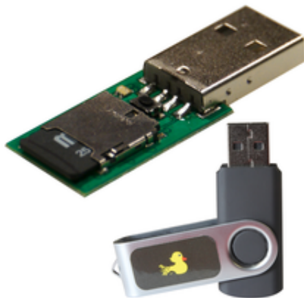
Figure 1: clé USB Rubber Ducky
